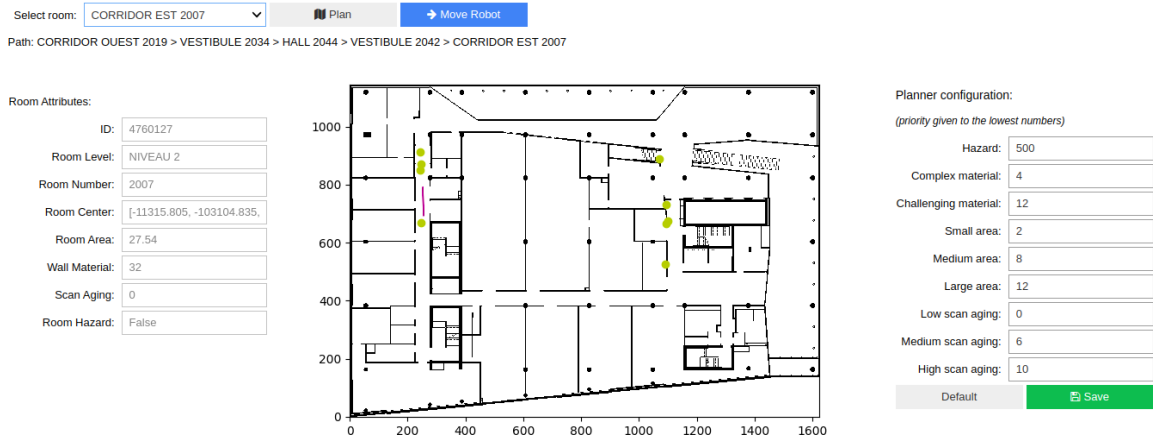
Figure 3. Semantic GUI for the intuitive operation of the robot navigation on construction sites. The controls in the header allow selecting a destination and generating the path. The panel to the left shows the attributes of the selected room. The center contains a map of the environment, with the robot's pose in real time represented by the purple arrow. The center points of the rooms and doors in the path are represented in the map by the yellow circles. The right panel allows the user to reconfigure the different weights applied to the path generation.
